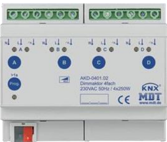
The Dimming Actuator (AKD-0401.02) is optimised for dimmable LED lights and can switch 250 W on each channel. Parallel operation of two channels with 500 W total power output is possible.
